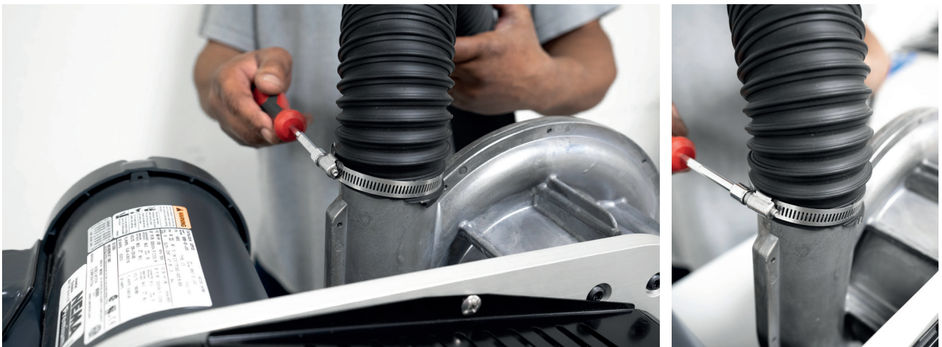
19. Reinstall connection to air delivery devices.
